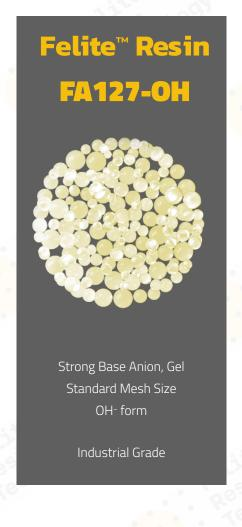
Felite™ FA127-OH is a high capacity, shock resistant, gel, Type I, strong base anion exchange resin supplied in hydroxide form, with both high operating capacity and the ability to achieve low residual silica levels.
