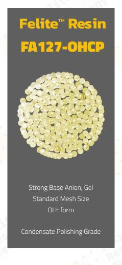
Felite™ FA127-OHCP is a polisher grade type I gel strong base anion resin with uniform mesh beads range, supplied in hydroxide form. It is specifically designed for use in deep bed condensate polishers and optimized both for low pressure loss and for perfect separation from the polisher grade cation components.
