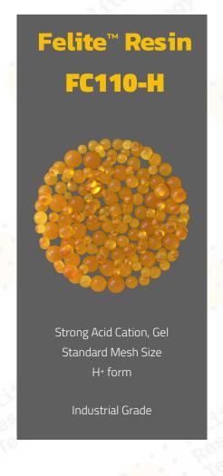
Felite™ FC110-H is a 10% crosslinked gel strong acid cation resin with standard mesh size range, supplied in hydrogen form. It is primarily used in the cation stage of demineralization plants use in industrial water treatment employing coflow regeneration. Its standard beads size distribution gives optimum operating capacity with minimum leakages of ions and also minimum pressure drop across the resin bed.
