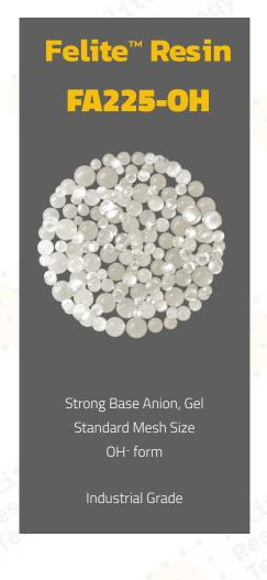
Felite™ FA225-OH is a type II gel strong base anion resin in hydroxide form. It has lower selectivities and therefore higher chemical efficiency and better resistance to fouling than type I anion resins. Their thermal sensitivity can result in reduced life when operating temperatures exceed 95°F.
